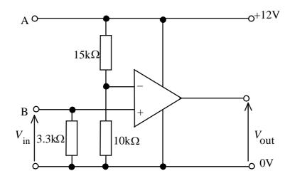
(a) Calculate the switching level of the comparator.
