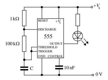
(a) Calculate the value of C needed to give a frequency of 1 kHz.
