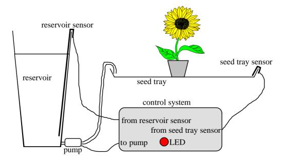
If the seed tray sensor is dry (logic 1) then the pump must be turned on (logic 1) until the seed tray sensor is wet (logic 0). If the reservoir sensor is dry (logic 1) because the reservoir is empty, then the warning LED must be illuminated (logic 1) but the pump must not be turned on even if the seed tray is dry.
